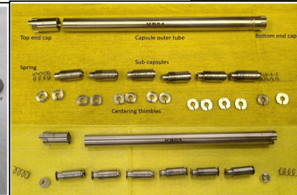
Irradiation Targets with Sub-Capsules
