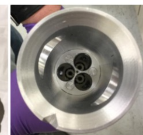
Basket Assembly with Irradiation Targets
